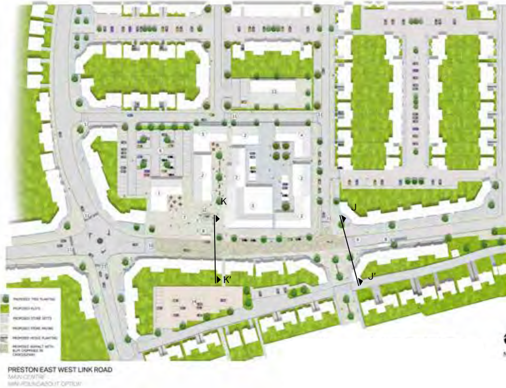
Fig 3.40 Diagram showing the desired materials and treatments for the Main Centre area with a mini roundabout configuration.
