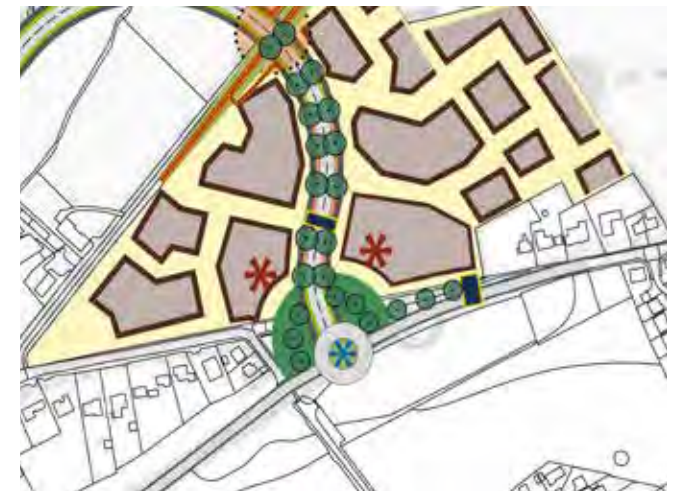
Fig 2.19 Eastern gateway : roundabout with landscape and building reinforcing the circular configuration
