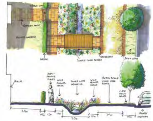
Fig 2.21 Illustrative diagram showing a potential incorporation of SUDS alongside the EWLR as well as material treatments and planting scheme
