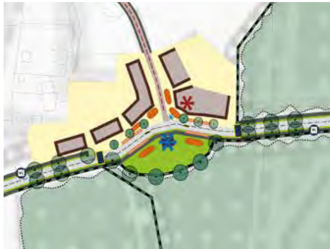
Fig 2.5 EWLR with a deflection aiming to reduce speeds
