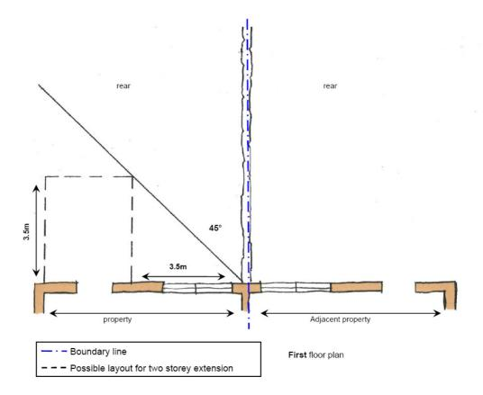
On a detached property no part of a two storey extension should cross the point at which a 45<sup>°</sup> line in the horizontal plane is drawn from the nearest part of a window to a habitable room on the immediately adjacent dwelling.
