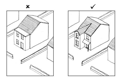
On semi-detached properties or terraced properties with gardens two storey extensions must be a minimum of 2 metres from the adjoining house.
