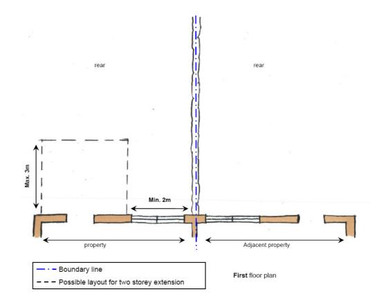
For extensions longer than 3 metres, the distance between the boundary of the adjoining property and the first floor element of the extension must be equidistant (i.e. the distance must be same or greater than the projection of the extension).
