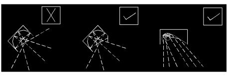
will also be beneficial to use as high a mounting height as possible, giving due regard to the daytime appearance of the installation. The requirements to control glare for the safety of road users are given in Table 2.
