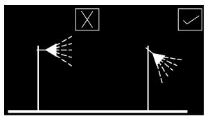
Use specifically designed lighting equipment that minimises the upward spread of light near to and above the horizontal. Care should be taken when selecting luminaires to ensure that appropriate units are chosen and that their location will reduce spill light and glare to a minimum. Remember that lamp light output in LUMENS is not the same as lamp wattage and that it is the former that is important in combating the problems of obtrusive light
